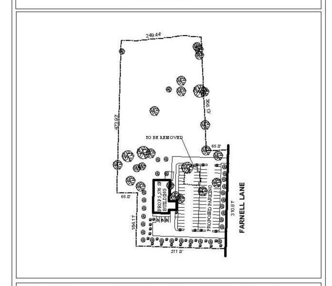
The site is located on the West side of Farnell Lane, 148' North of Pleasant Valley Road, extending West to the East terminus of Angus Drive and Kendale Drive. The plan illustrates the existing structure to be removed, along with the proposed structure and parking.
