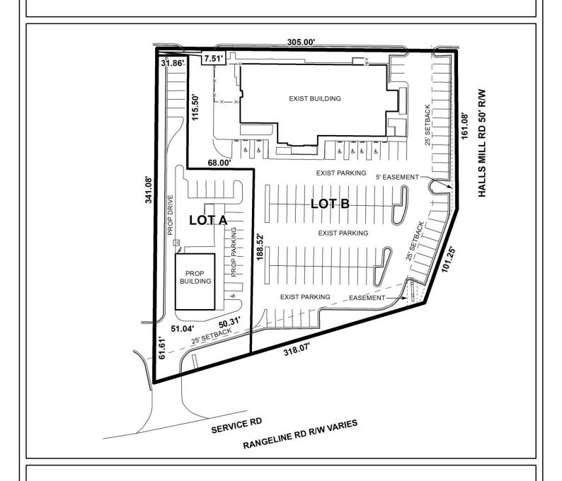
The site plan illustrates the existing building, existing parking, setbacks, easements, proposed building, and proposed parking.
