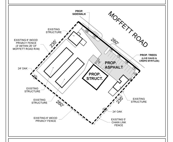
The site is located on the South side of Moffett Road at Pine Grove Avenue. The plan illustrates the existing and proposed structures, paving and trees.
