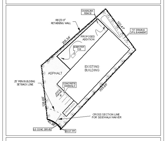
Existing buildings, parking, easements, setbacks, and the proposed addition and cross section line for sidewalk waiver are illustrated in the site plan.
