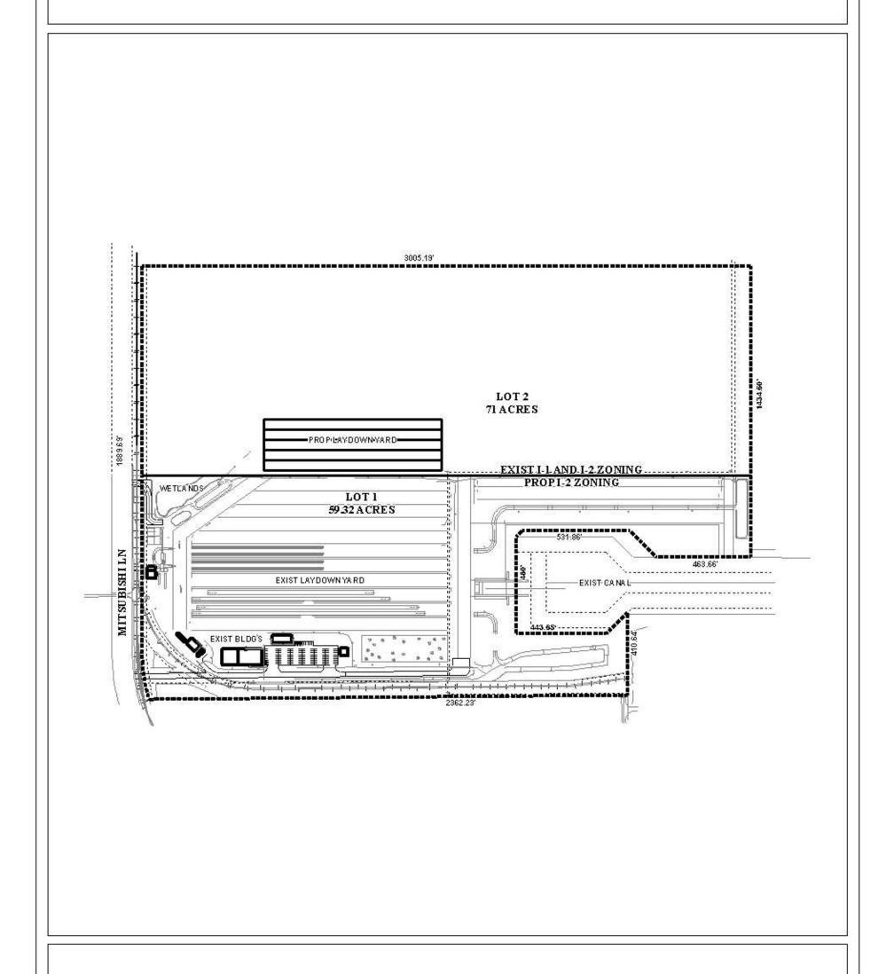
The site plan illustrates the existing concrete manufacturing facility and proposed laydown yard.
