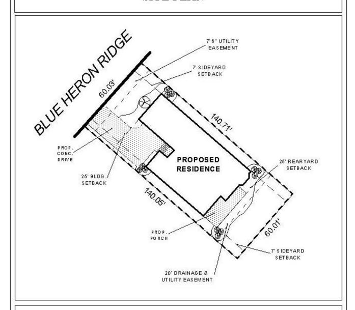
The site is located on the South side of Blue Heron Ridge, 320' West of its East terminus. The plan illustrates the proposed structure, setbacks and easements.
