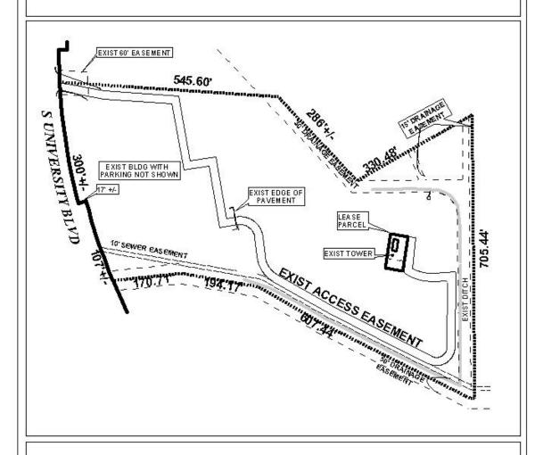
The site plan illustrates the existing drainage and sewer easements, building, and tower along with the existing access easements and lease parcel.
