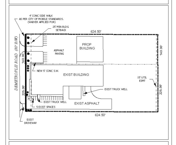
The site plan illustrates existing buildings, parking and drive, proposed parking and building, and proposed sidewalk.
