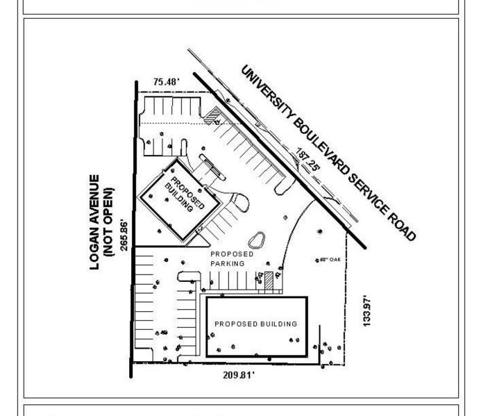
The site is located on the West side of University Boulevard, 615' North of Zack Logan Avenue North, Extending to the East side of Logan Avenue. The plan illustrates the proposed structures and parking.
