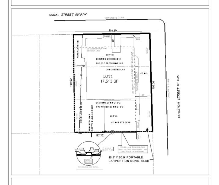
The site plan illustrates the existing lot configuration, existing and proposed zoning, and location of structures.
