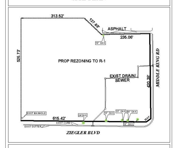
The site plan illustrates the existing landscaping, sewer, drainage, and utility structures.
