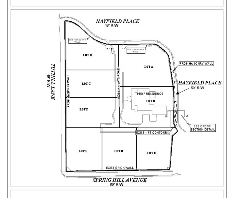
The site plan illustrates the existing lot configuration, proposed masonry wall, and existing walls.
