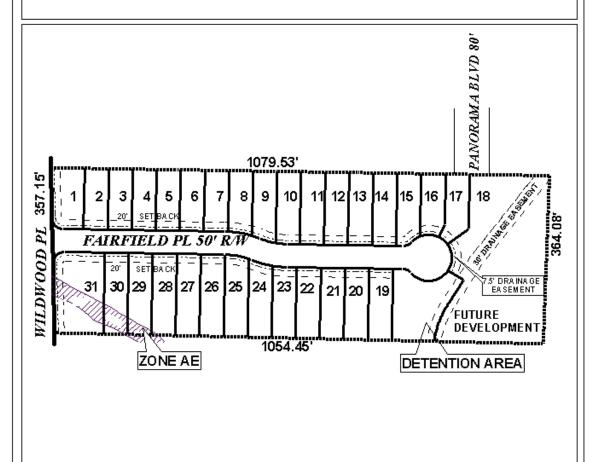
The site plan illustrates the lot configuration, proposed setbacks, easements, detention areas, and existing floodways.
