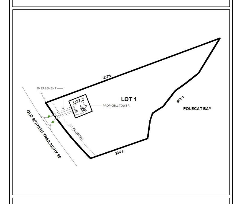
The site plan illustrates the easements and propsoed cell tower location.
