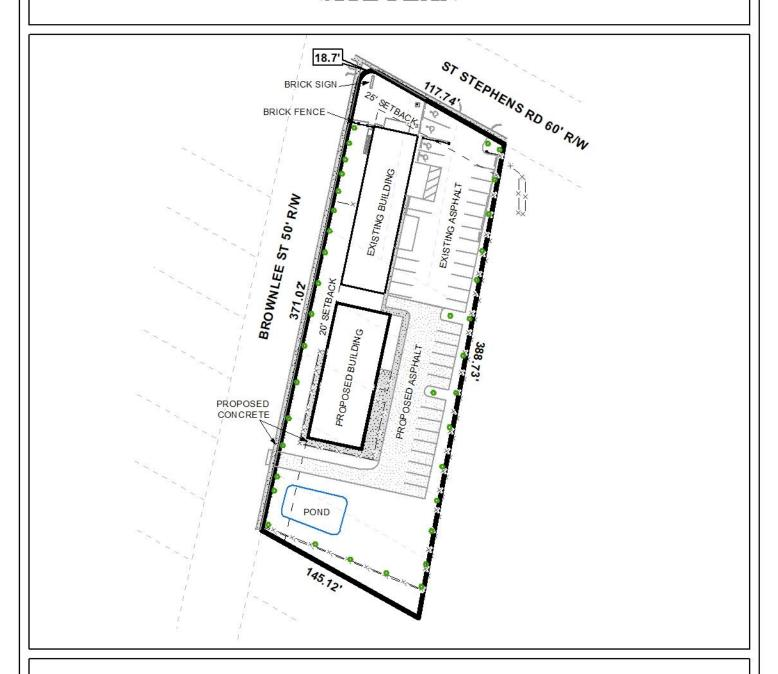
The site plan illustrates existing structures, surfaces, setbacks and proposed strutures, surfaces and detention pond.
