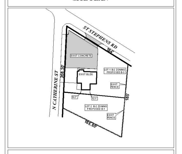
The site plan illustrates the existing building, fencing, and concrete.
