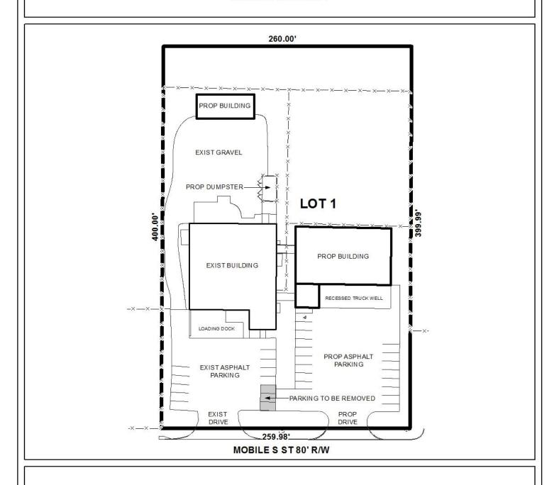
The site plan illustrates the existing building, existing parking, existing drive, proposed buildings, proposed parking, and proposed drive.
