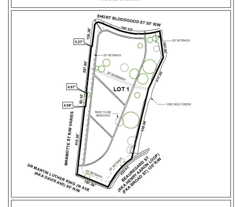
The site plan illustrates the easement, setbacks, and trees to be removed.
