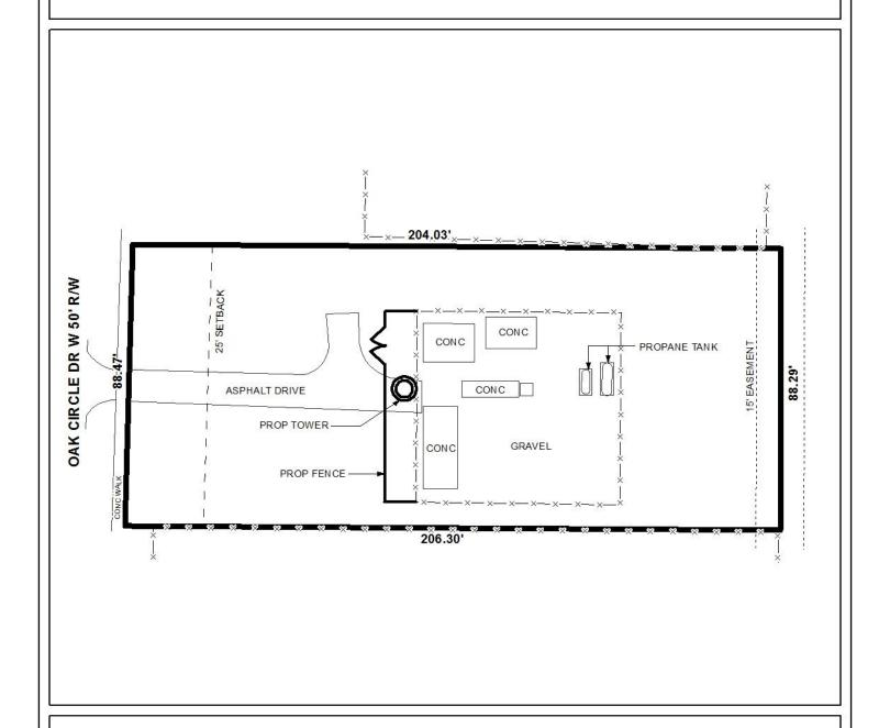
The site plan illustrates the proposed tower, proposed fence, asphalt drive, setback, and easement.
