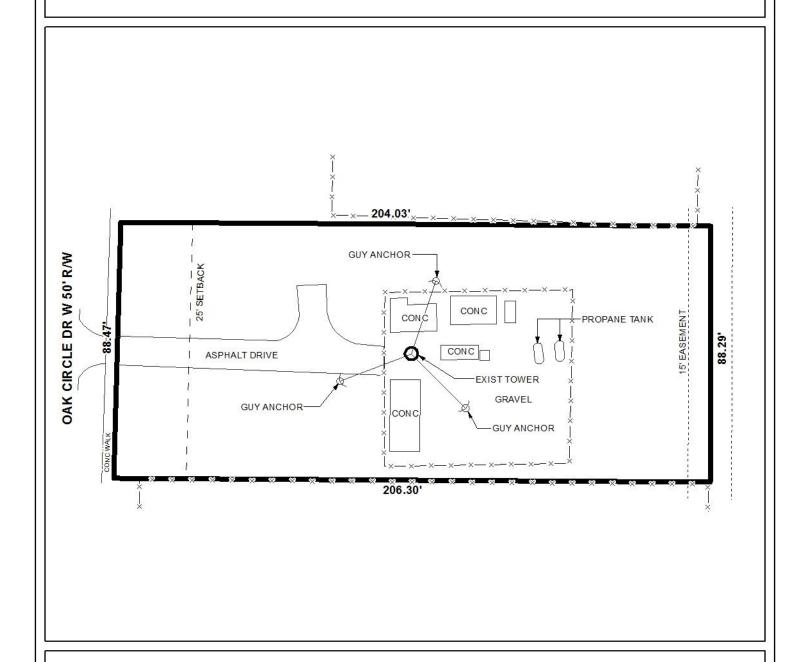
The site plan illustrates the existing tower, asphalt drive, setback, and easement.
