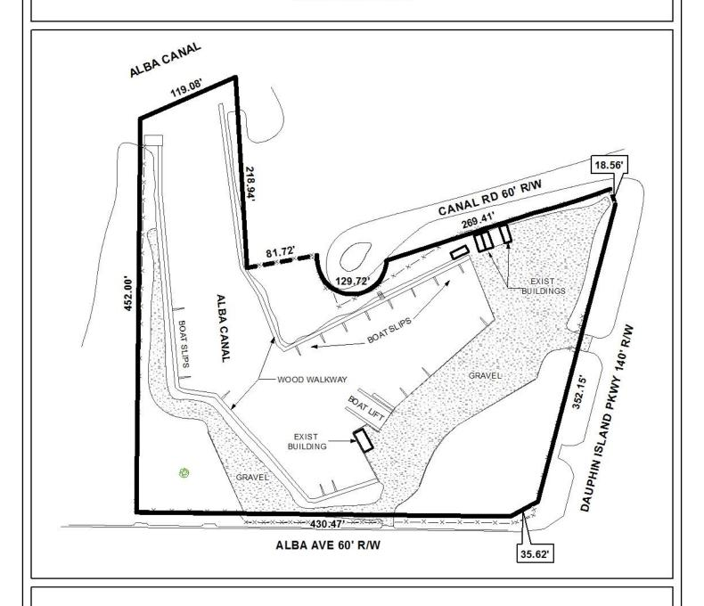
The site plan illustrates the existing buildings, existing boat slips, existing walkways, and existing gravel area.
