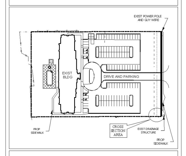
The site plan illustrates existing building, parking, drive, proposed sidewalks and location of power pole and guy wire.
