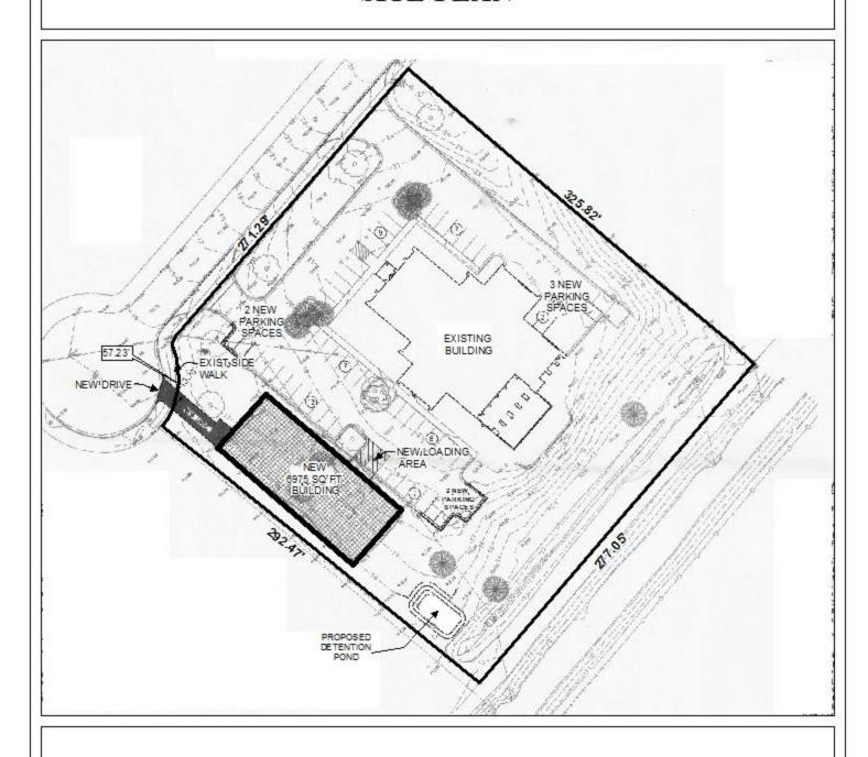
The site plan illustrates the existing building, the proposed building, new pond, new drive, and parking.
