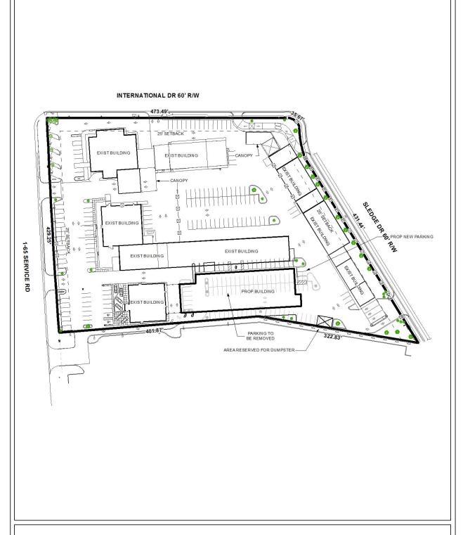
The site plan illustrates the proposed building under Phase 2, proposed parking, the existing buildings, and setbacks.
