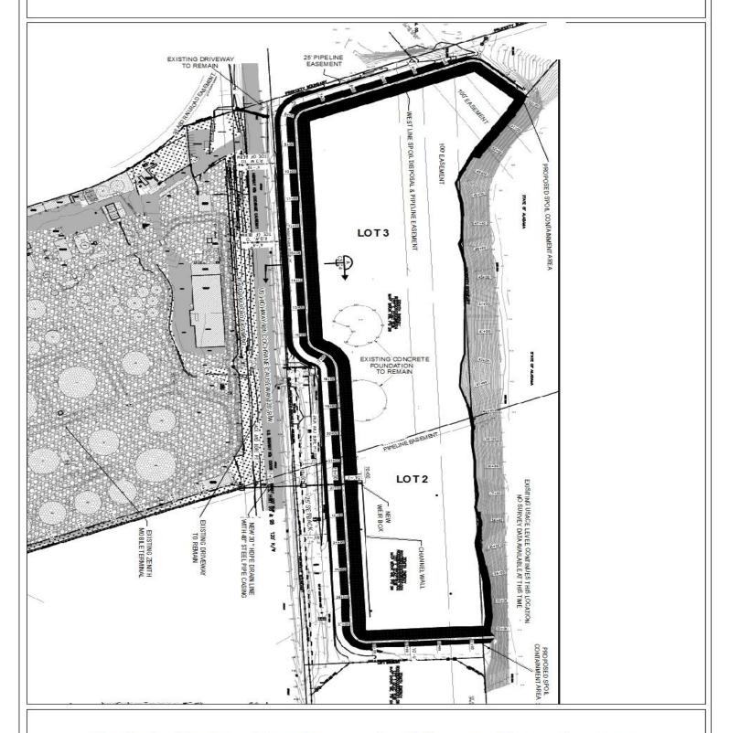
The site plan illustrates existing tanks, proposed spoil site, proposed berm, and easements.
