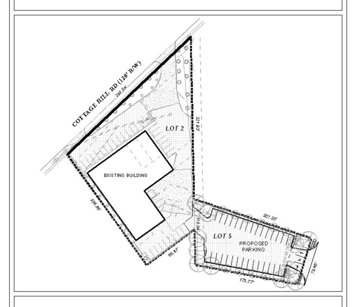
This site plan illustrates the existing building and proposed overflow parking.
