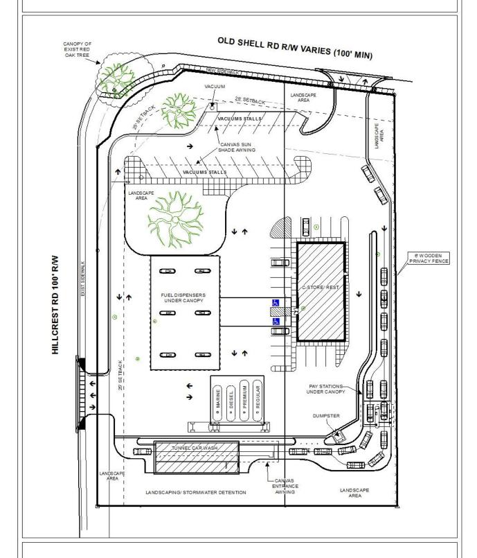
The site plan illustrates the proposed convenience store, new sidewalk, fuel tanks, canopies, and car wash area.
