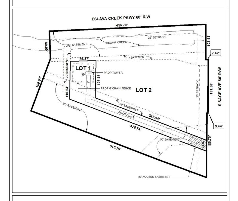
The site plan illustrates the easements, setbacks, proposed lots, proposed drive, and proposed tower location.
