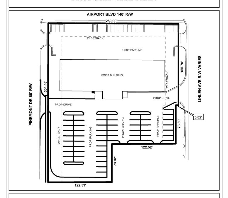
The site plan illustrates the existing building, existing parking, setbacks, proposed parking, and proposed drives.
