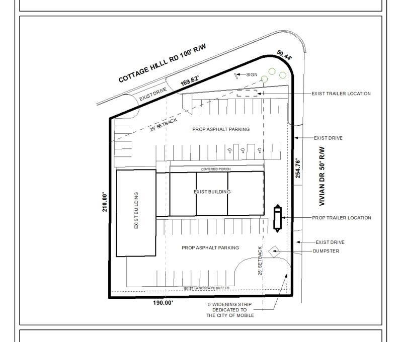
The site plan illustrates the existing buildings, existing drives, setbacks, easements, proposed parking, and proposed trailer location.
