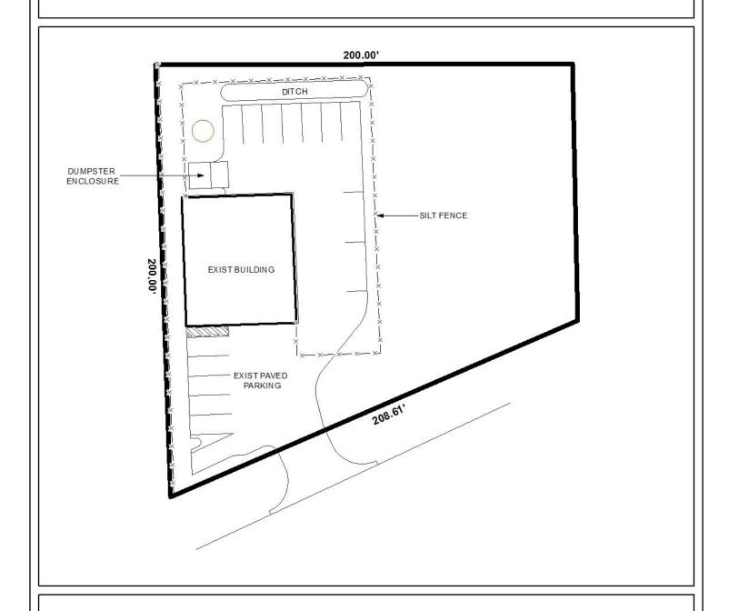
The site plan illustrates the existing building, ditch, and existing parking.
