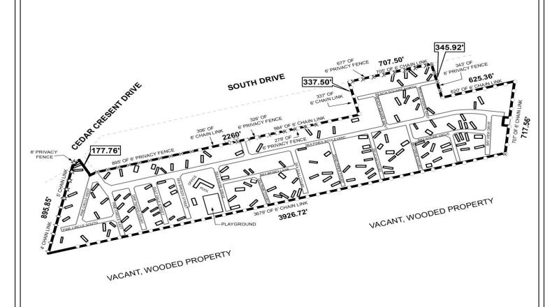
The site plan illustrates existing structures, fencing and right of ways.
