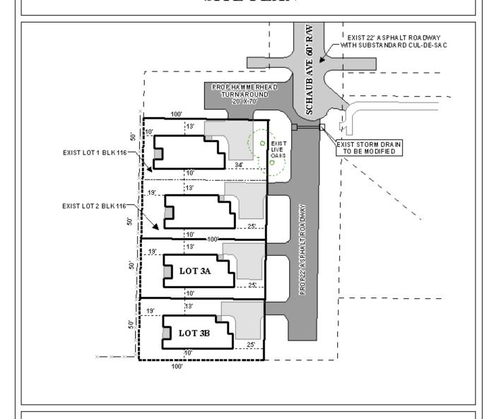
The site plan illustrates the proposed lot configuration, proposed residential structures, setbacks, and proposed asphalt road.
