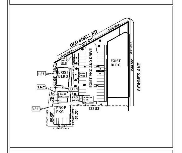
The site plan illustrates the existing buildings to remain and to be removed, existing parking, easement, along with proposed parking, drives, and resubdivision
