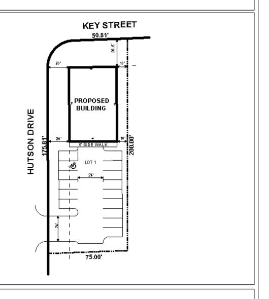
The site is located on the Southeast corner of Hutson Drive and Key Street. The plan illustrates the proposed structure and parking.
