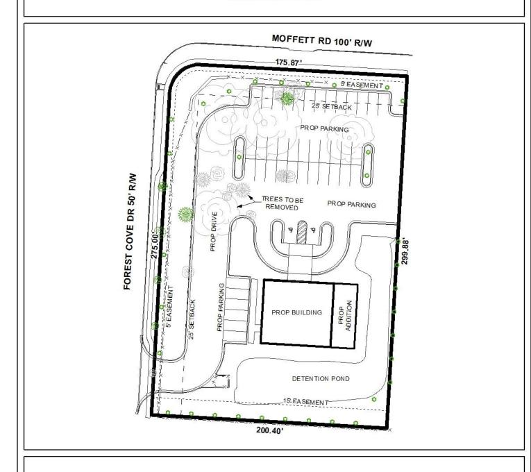
The site plan illustrates the proposed building, proposed parking, setbacks, easements, trees to be removed, and detention pond.
