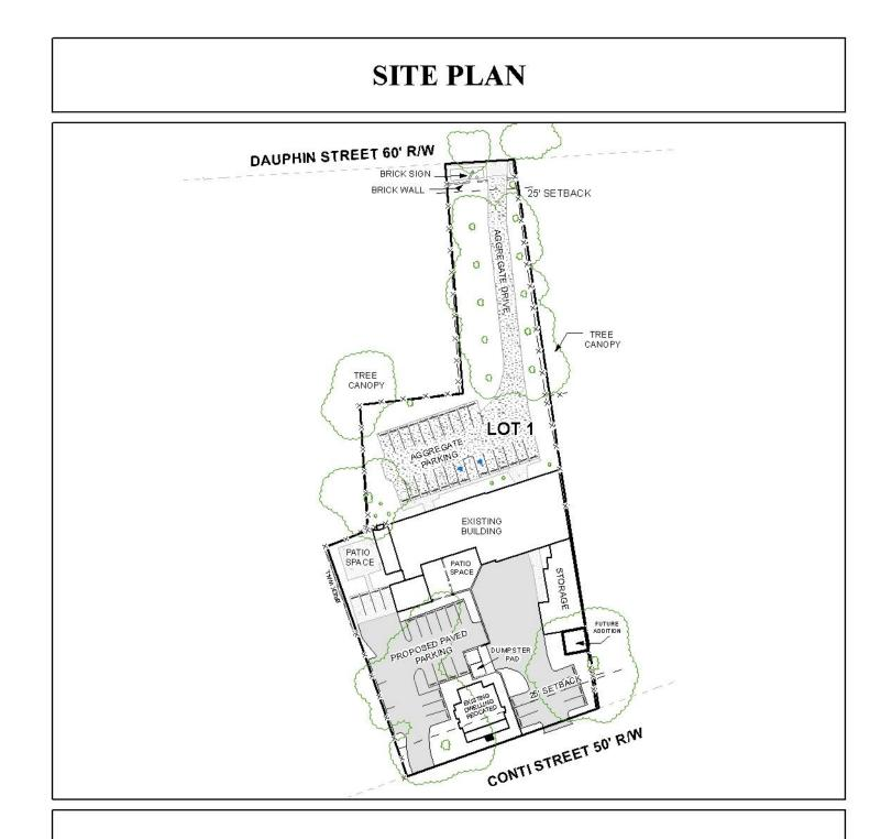
The site plan illustrates exisiting buildings, aggregate parking, and setback. As well as existing storage area with future addition, and proposed paved parking area.
