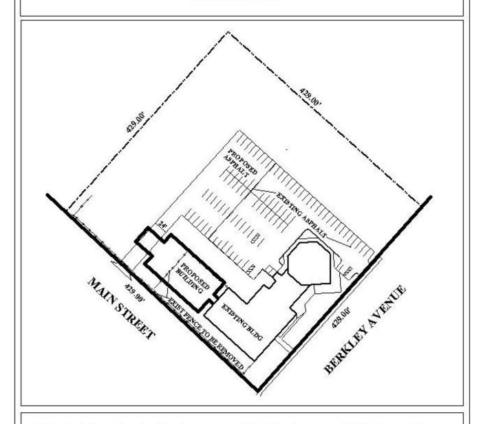
The site is located on the Northeast corner of Berkley Avenue and Main Street. The plan illustrates the existing structure and parking, along with the proposed building and parking.
