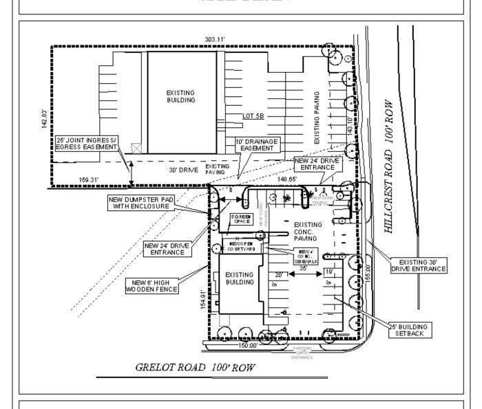
The site plan illustrates the existing and proposed drives, joint ingress/egress, and parking.
