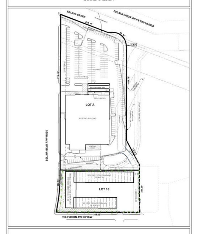
The site plan illustrates the existing building, parking, proposed building, and parking, setbacks, and easements.
