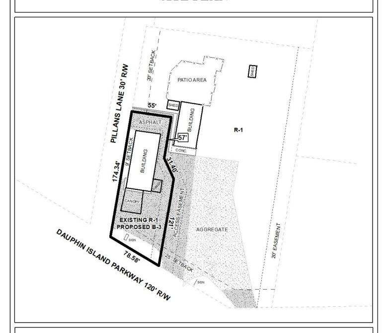
The site plan illustrates existing buildings, setbacks, easements and surfaces. As well as existing and proposed zoning.
