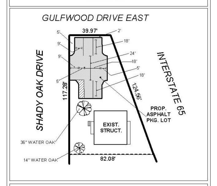
The site is located at the Southeast corner of Shady Oak Drive and Gulfwood Drive East, extending to the West I-65 Service Road North. The plan illustrates the existing structure and proposed parking.
