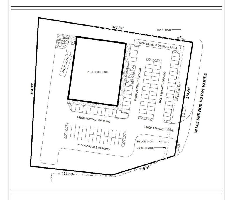
The site plan illustrates the proposed building, proposed drive, proposed asphalt parking, and setback.
