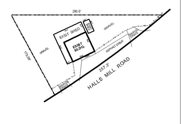
The site is located on the North side of Halls Mill Road, 120' West of the North terminus of Riviere Du Chien Road. The plan illustrates the existing buildings, drives, and fencing.
