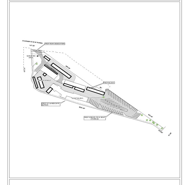
$The \ site \ plan \ illustrates \ the \ existing \ structures, proposed \ structures, and \ proposed \ RV \ and \ bo \ at \ storage \ area.$
