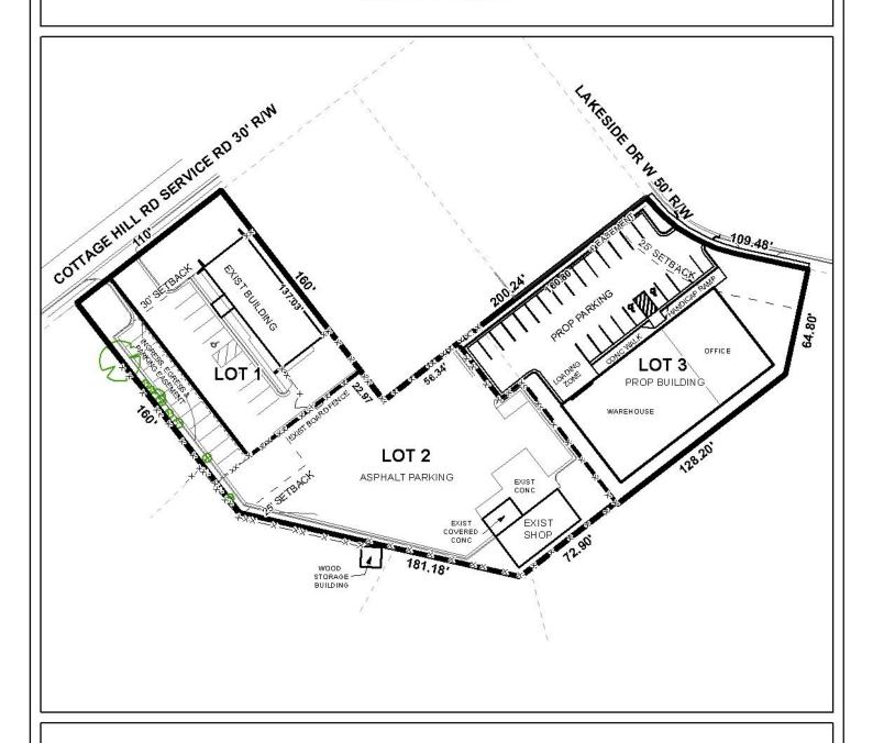
The site plan illustrates the existing buildings, proposed building, proposed parking, setbacks, and easements.
