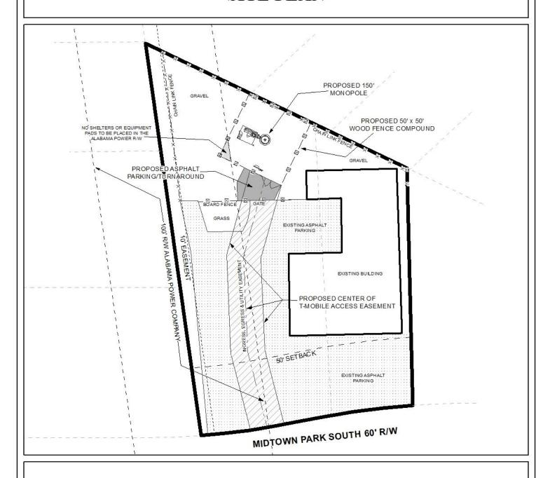
The site plan illustrates the proposed monopole, the proposed fences, proposed parking, the existing building, setbacks and easements.
