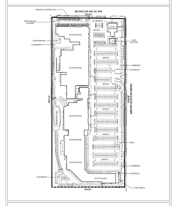
The site plan illustrates the existing buildings, existing parking facility, setbacks, easements, proposed parking changes, and proposed drive.
