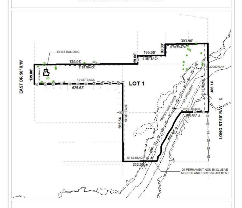
The site plan illustrates the existing building, setbacks, easements, and floodzones.
