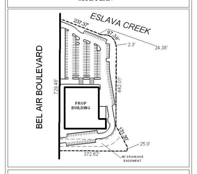
The site is located on the East side of Bel Air Boulevard, 210'north of Television Avenue, extending North to the South side of Eslava Creek. The plan illustrates the proposed structure and parking.
