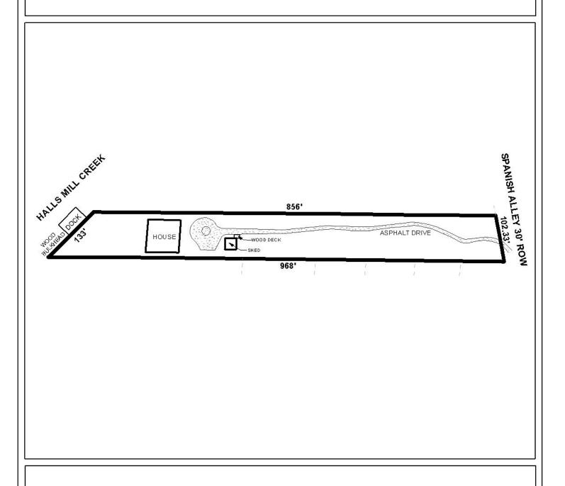
The site plan illustrates proposed structures and asphalt drive.
